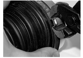
Step 4 Place the clamp over object. Engage interlocking hooks in tightest window position. Firmly crimp the ear with Oetiker pincers.
