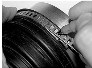
Step 2 Determine the clamp length.
