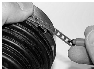
Step 2 Determine the clamp length. Make sure the end of the clamp passes the "ear", as shown.
